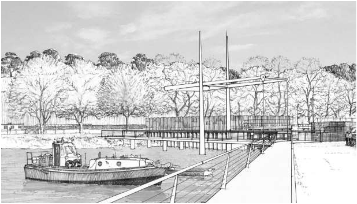
Figure 32: Illustration of a lifting bascule option hinged from Boscawen Park side (Produced by Yee Associates for Hewson Engineering)
