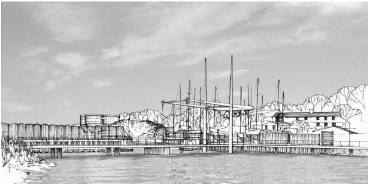
Figure 33: Illustration of a lifting bascule option hinged from Lighterage Quay side (Produced by Yee Associates for Hewson Engineering)
