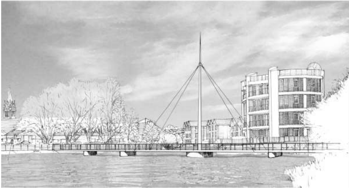
Figure 30: Illustration of a lifting bascule option with mast at Garras Wharf (Produced by Yee Associates for Hewson Engineering)
