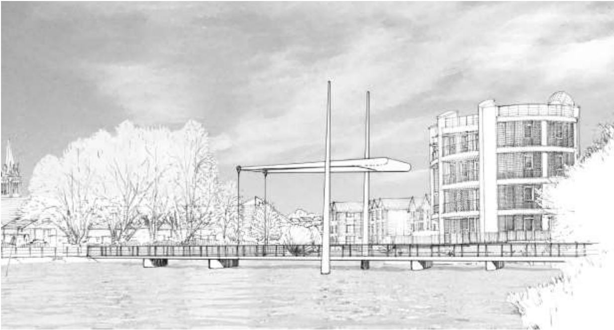
Figure 34: Illustration of a lifting bascule option at Garras Wharf (Produced by Yee Associates for Hewson Engineering)
